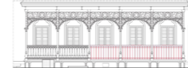
Example of using Alternate Repair material & Technique Case of Cast Iron railing completed using GI railing for the missing units
