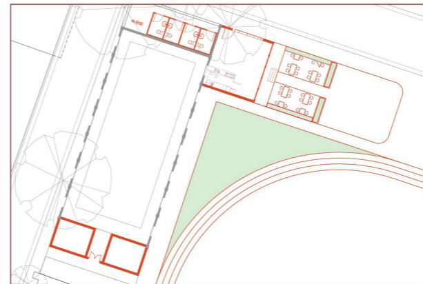
Plan of Kumartuli Swimming pool with new opening and later additions of toilet block and cafe
